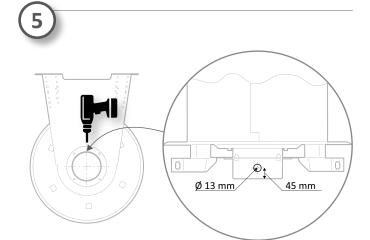
5. Drill a hole, Ø 13 mm, in the hose reel flange (5). Remove any sharp metal shavings from the hole.
