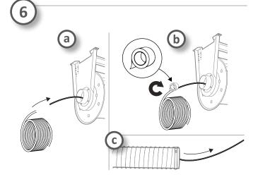
Fasten the compressed air hose to the string (6a-b). Then use the string to pull the compressed air hose through the exhaust hose.
