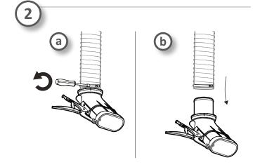
2. If an exhaust nozzle is fitted to the extraction hose, detach the exhaust nozzle to free the end of the extraction hose (2a-b).
