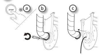
4. Stop the fan (4a) and detach the hose or spiro duct from the hose reel outlet (b-c).
