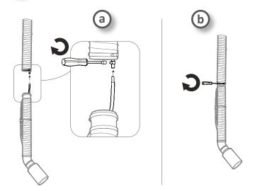
8. Connect the compressed air hose in the extraction hose with the one in the exhaust nozzle (8a). Attach the exhaust nozzle (b).
