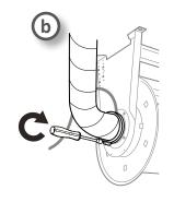
10. Attach the hose/spiro duct to the hose reel outlet (10a-b).
