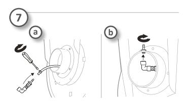
7. Attach the compressed air hose to the compressed air fitting (7a). Then fit the threaded nipple with the fitting through the hole you drilled in the hose reel flange (b).
